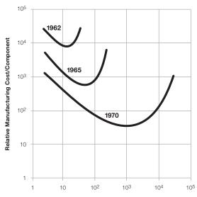
Number of Components Per Integrated Circuit
